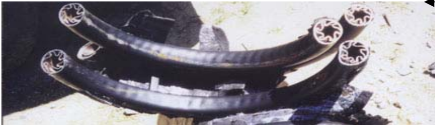
Cu-Ni 706 Alloy Water Tube Fluted HX in Steel Refrigerant Outer Tube
